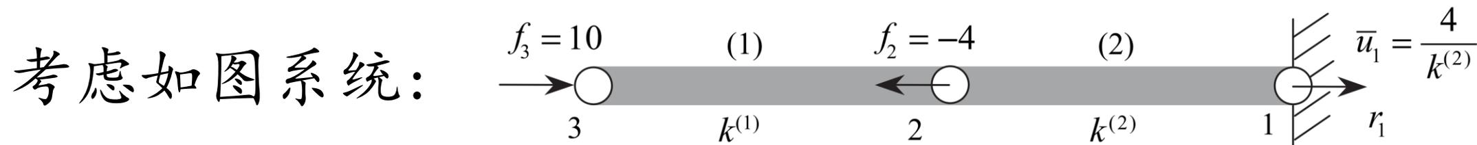
$$\begin{bmatrix} \mathbf{K}_E & \mathbf{K}_{EF} \\ \mathbf{K}_{EF}^T & \mathbf{K}_F \end{bmatrix} \begin{bmatrix} \bar{\mathbf{d}}_E \\ \mathbf{d}_F \end{bmatrix} = \begin{bmatrix} \mathbf{r}_E \\ \mathbf{f}_F \end{bmatrix}$$
