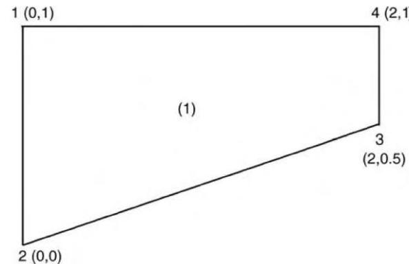
$$\mathbf{f}_{\Gamma}^e = \int_{\Gamma_{14}} (\mathbf{N}^{4Q})^T \bar{\mathbf{t}} d\Gamma = \int_{\eta=-1}^1 (\mathbf{N}^{4Q})^T (\xi = -1, \eta) d\eta \bar{\mathbf{t}} = \begin{bmatrix} 1 & 0 \\ 0 & 1 \\ 0 & 0 \\ 0 & 0 \\ 0 & 0 \\ 0 & 0 \\ 1 & 0 \\ 0 & 1 \end{bmatrix} \begin{bmatrix} 0 \\ -20 \end{bmatrix} = \begin{bmatrix} 0 \\ -20 \\ 0 \\ 0 \\ 0 \\ 0 \\ 0 \\ -20 \end{bmatrix}$$
