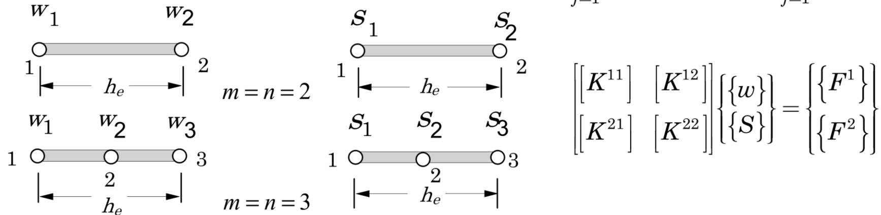
$$K_{ij}^{11} = \int_{x_a}^{x_b} \left( GAK_s \frac{d\psi_i}{dx} \frac{d\psi_j}{dx} + c_f \psi_i \psi_j \right) dx, \quad K_{ij}^{12} = \int_{x_a}^{x_b} GAK_s \frac{d\psi_i}{dx} \varphi_j dx = K_{ji}^{21}$$
