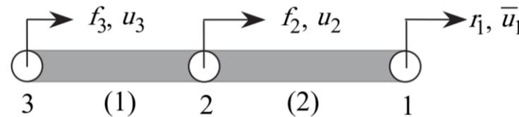
$$\mathbf{d}^{(1)} = \begin{bmatrix} u_1^{(1)} \\ u_2^{(1)} \end{bmatrix} = \underbrace{\begin{bmatrix} 0 & 0 & 1 \\ 0 & 1 & 0 \end{bmatrix}}_{\mathbf{L}^{(1)}} \begin{bmatrix} \bar{u}_1 \\ u_2 \\ u_3 \end{bmatrix} = \mathbf{L}^{(1)} \mathbf{d},$$
