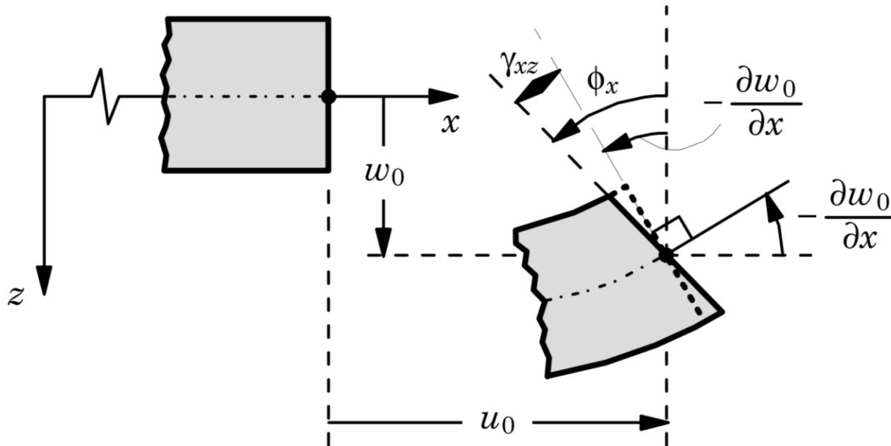
The classical plate theory underpredicts deflections and overpredicts frequencies as well as buckling loads of plates with side-to-thickness ratios of the order of 20 or less (i.e., thick plates). 对厚板使用 Kirchhoff板理论会低估挠度，并且高估频率和屈曲荷载。
