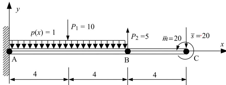
$$\mathbf{f}_{\Gamma}^e = (\mathbf{N}^{eT} \bar{s})|_{\Gamma_s} + \left( \frac{d\mathbf{N}^{eT}}{dx} \bar{m} \right) |_{\Gamma_m}$$
