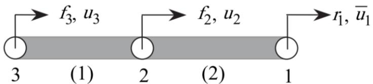
$$\underbrace{\begin{bmatrix} 0 \\ F_2^{(1)} \\ F_1^{(1)} \end{bmatrix}}_{\tilde{\mathbf{F}}^{(1)}} + \underbrace{\begin{bmatrix} F_2^{(2)} \\ F_1^{(2)} \\ 0 \end{bmatrix}}_{\tilde{\mathbf{F}}^{(2)}} = \begin{bmatrix} r_1 \\ f_2 \\ f_3 \end{bmatrix} = \underbrace{\begin{bmatrix} 0 \\ f_2 \\ f_3 \end{bmatrix}}_{\mathbf{f}} + \underbrace{\begin{bmatrix} r_1 \\ 0 \\ 0 \end{bmatrix}}_{\mathbf{r}}$$
