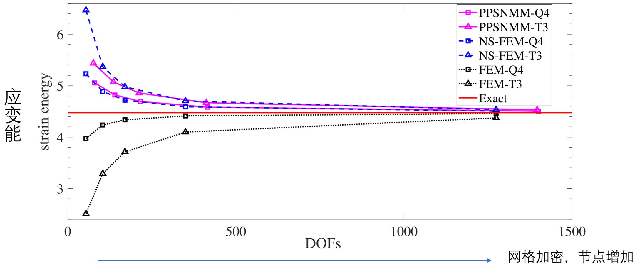
Figure 13: Strain energies of the cantilever obtained with different methods.
