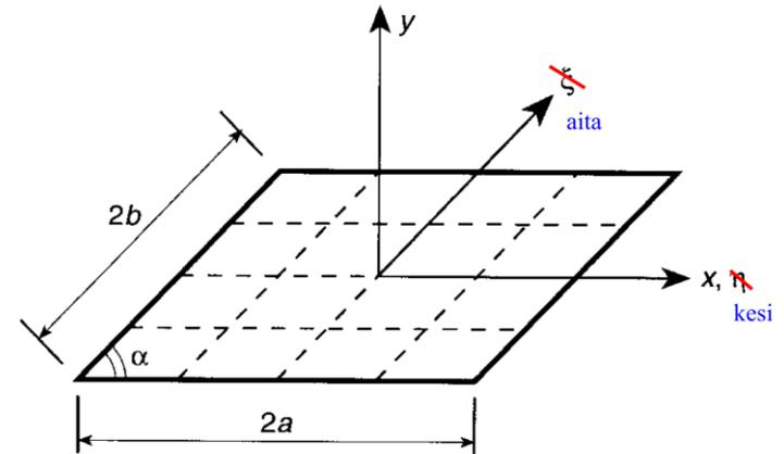
It will be observed that the gradient of  $w$  normal to any of the boundaries also varies along it in a cubic way. (Consider, for instance, values of the normal  $\partial w / \partial x$  along a line on which  $x$  is constant.) As on such lines only two values of the normal slope are defined, the cubic is not specified uniquely and, in general, a discontinuity of normal slope will occur. The function is thus ‘non-conforming’.
