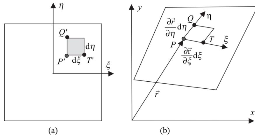
Mapping of the infinitesimal areas from (a) the parent domain to (b) the physical domain.
