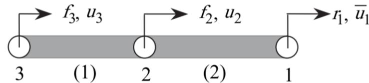
$$\underbrace{\begin{bmatrix} 0 \\ F_2^{(1)} \\ F_1^{(1)} \end{bmatrix}}_{\tilde{\mathbf{F}}^{(1)}} + \underbrace{\begin{bmatrix} F_2^{(2)} \\ F_1^{(2)} \\ 0 \end{bmatrix}}_{\tilde{\mathbf{F}}^{(2)}} = \begin{bmatrix} r_1 \\ f_2 \\ f_3 \end{bmatrix} = \underbrace{\begin{bmatrix} 0 \\ f_2 \\ f_3 \end{bmatrix}}_{\mathbf{f}} + \underbrace{\begin{bmatrix} r_1 \\ 0 \\ 0 \end{bmatrix}}_{\mathbf{r}} \quad \longrightarrow \quad \sum_{e=1}^2 \mathbf{L}^{eT} \mathbf{F}^e = \mathbf{f} + \mathbf{r}$$
