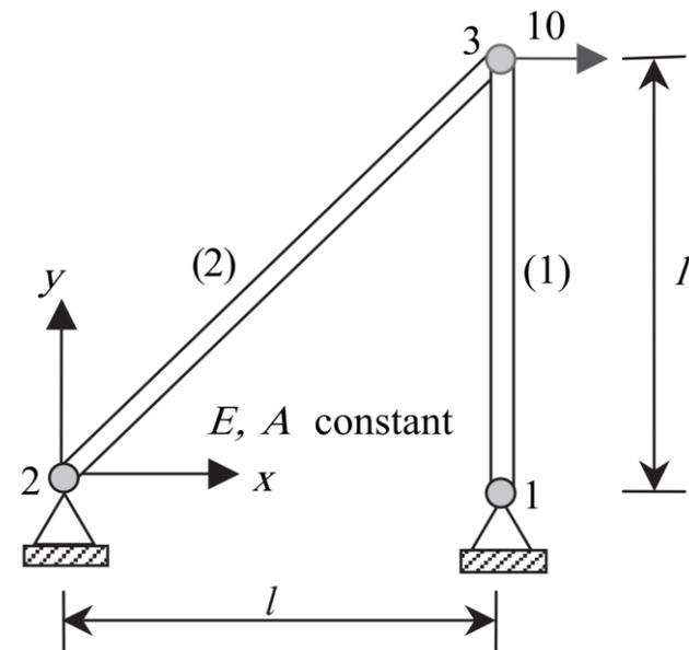
Figure 2.13 Two-element truss structure.
