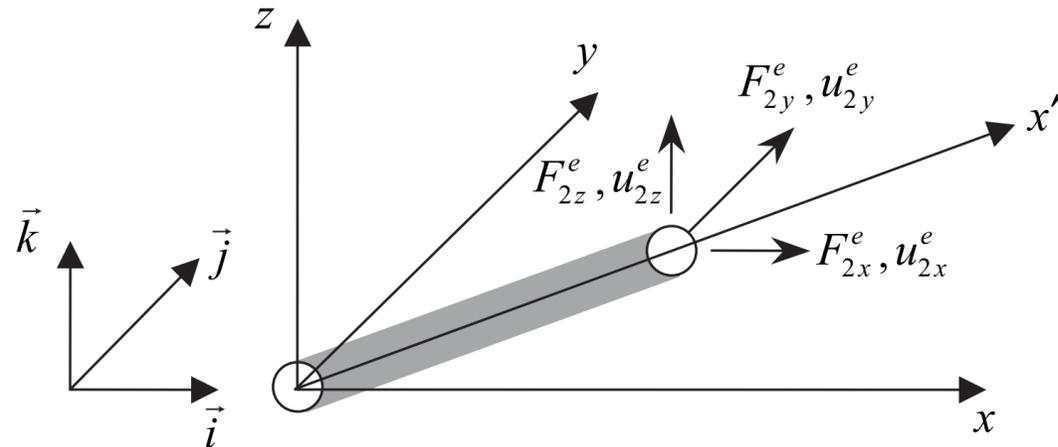
$$\mathbf{d}^e = [u_{1x}^e \quad u_{1y}^e \quad u_{1z}^e \quad u_{2x}^e \quad u_{2y}^e \quad u_{2z}^e]^T$$
