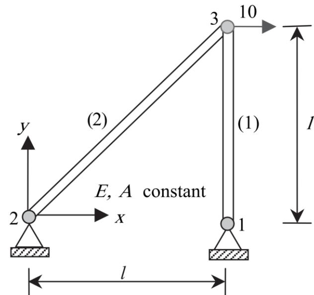
Figure 2.13 Two-element truss structure.
