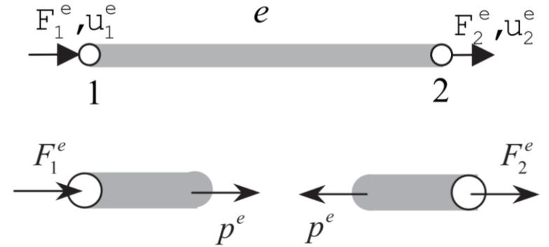
$$\begin{aligned} F_2^e &= p^e = A^e \sigma^e \\ &= A^e E^e \varepsilon^e \\ &= A^e E^e \frac{\delta^e}{l^e} \end{aligned}$$
