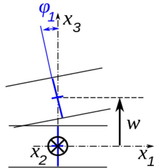
$$\begin{aligned}u(x, y, z, t) &= u_0(x, y, t) + z\phi_x(x, y, t) \\v(x, y, z, t) &= v_0(x, y, t) + z\phi_y(x, y, t) \\w(x, y, z, t) &= w_0(x, y, t)\end{aligned}$$
