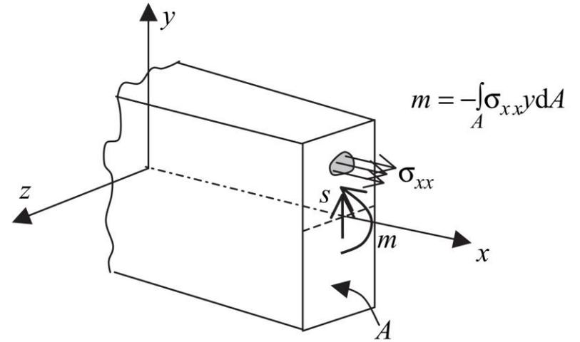
The resultant moment  $m$  and shear  $s$  on a cross section of the beam
