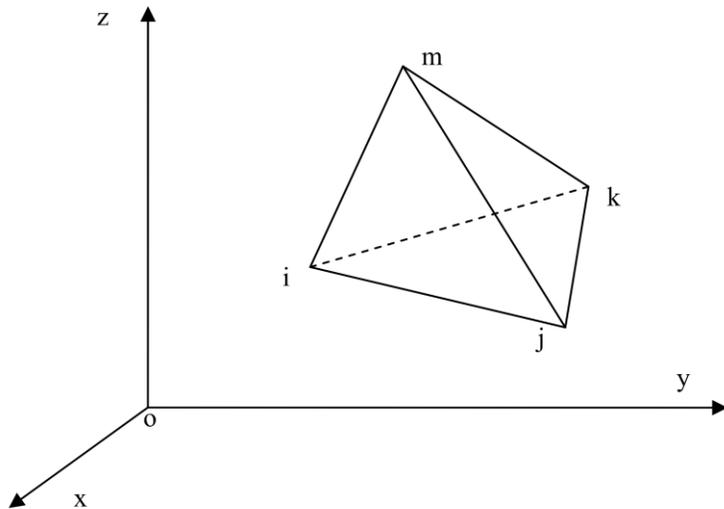
$$\{u\} = \begin{Bmatrix} u \\ v \\ w \end{Bmatrix} = \begin{Bmatrix} u(x, y, z) \\ v(x, y, z) \\ w(x, y, z) \end{Bmatrix}$$
