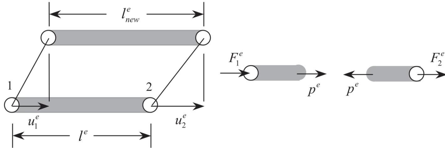
Figure 2.4 Elongation of an element and free-body diagrams, showing the positive sense of  $p^e$  and  $F_1^e$ .
