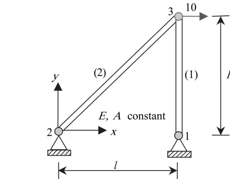
Figure 2.13 Two-element truss structure.
